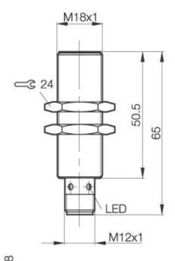
**Inductive Sensors BES M18MI-PSC50A-S04G-WM01** M18x1 x 65 normally-open Sn=5mm shielded
